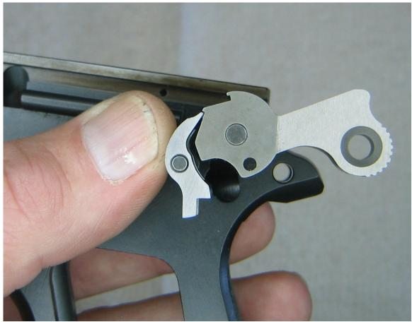
This is an NCO A2 model Sear on a model A1 Hammer. Pivot Sear, Hammer falls. Mil-Spec to memory is a 0.026 to 0.030" Sear ledge notch above.
