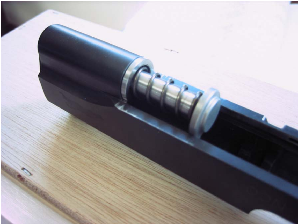
Reverse Plug Installed
