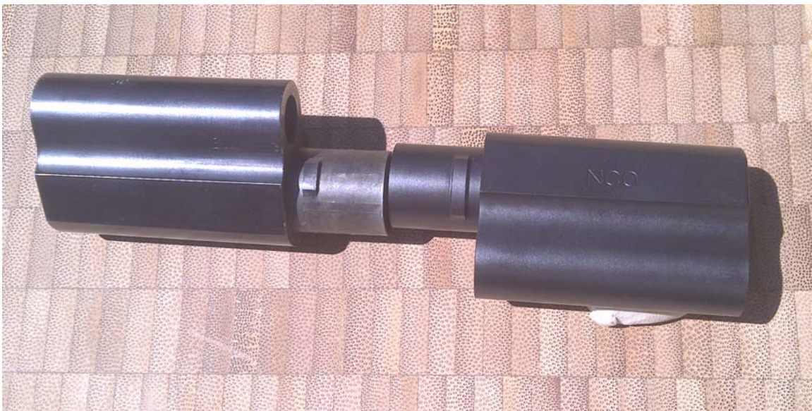
Note the T-1 connection lug on the right compared to one on a 1911 left
