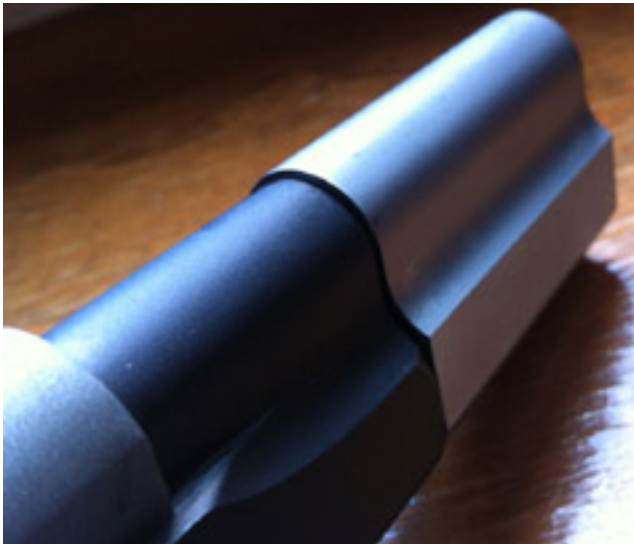
Fig. 1 "C" Model Compensator is larger than this 1911 Slide. It must be filed to match the slide of non-mil-spec Slides.
