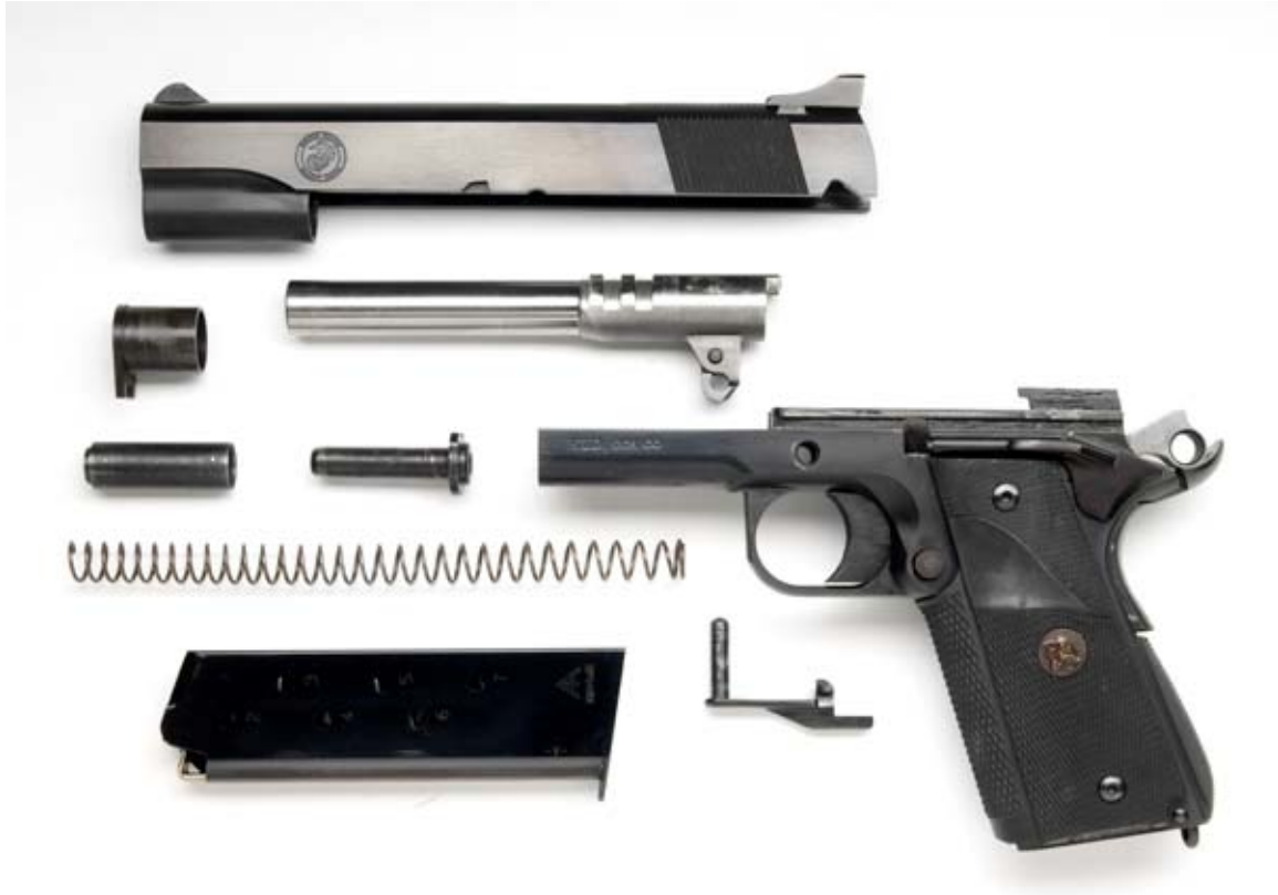
Fig. 8 Field Disassembly 1911 A2
