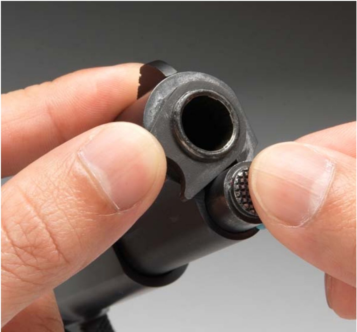
Figure 5. Remove the Recoil Spring Plug. Here shown is 1911 A2 plug.
