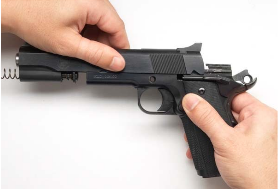
Fig. 7 Remove the Slide
