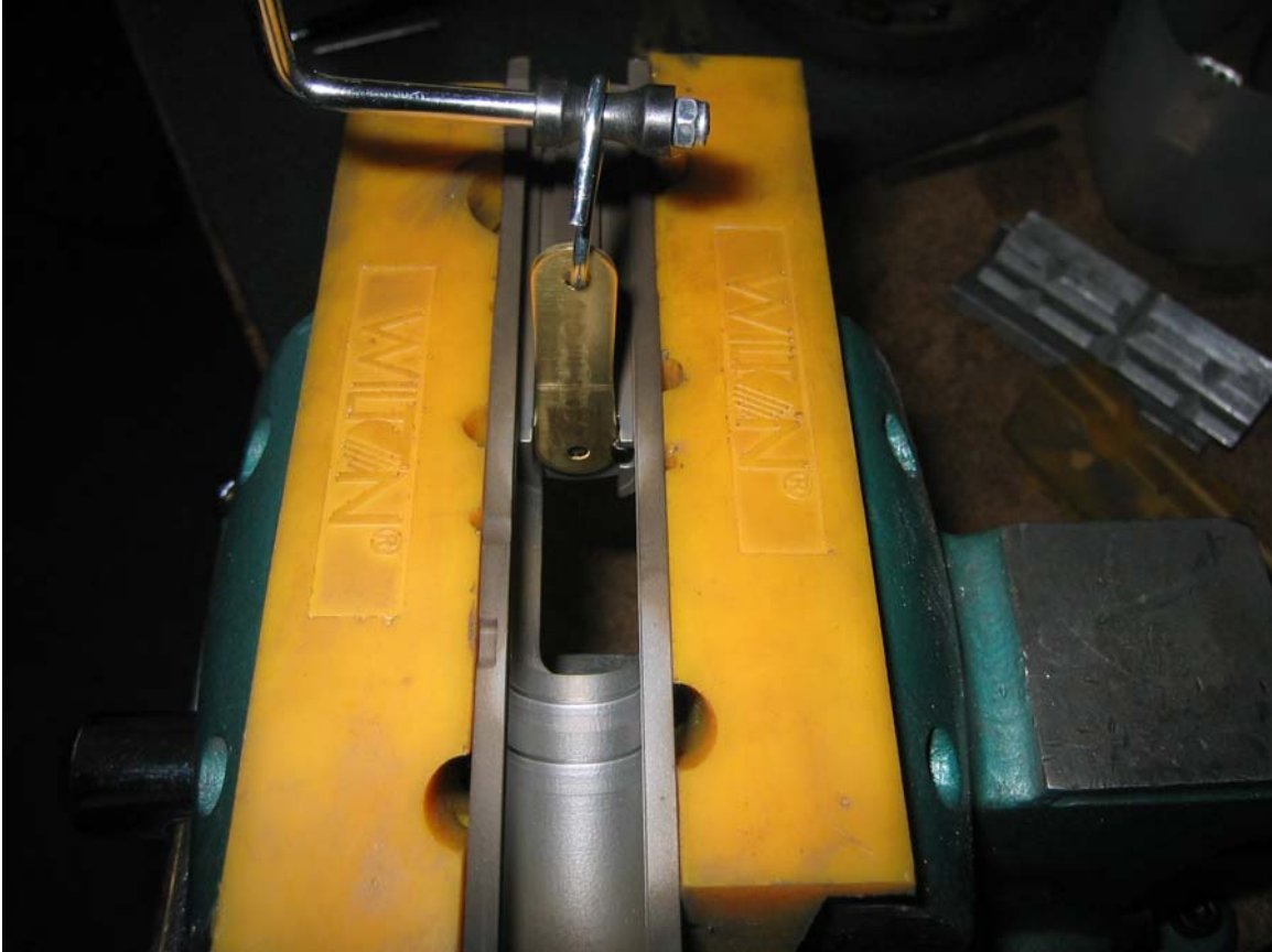
Combat NCO Extractor being weight tested using a pull gauge.
