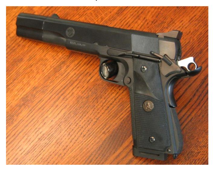
This is Serial Number KL3000 Combat NCO that at 3,000 rounds shot 400 yards open sight. At 5,000 rounds using bulk ammo shot 13" at 200 yards in a Ransom Rest shown elsewhere on this website under Testing. A borrowed gun.
