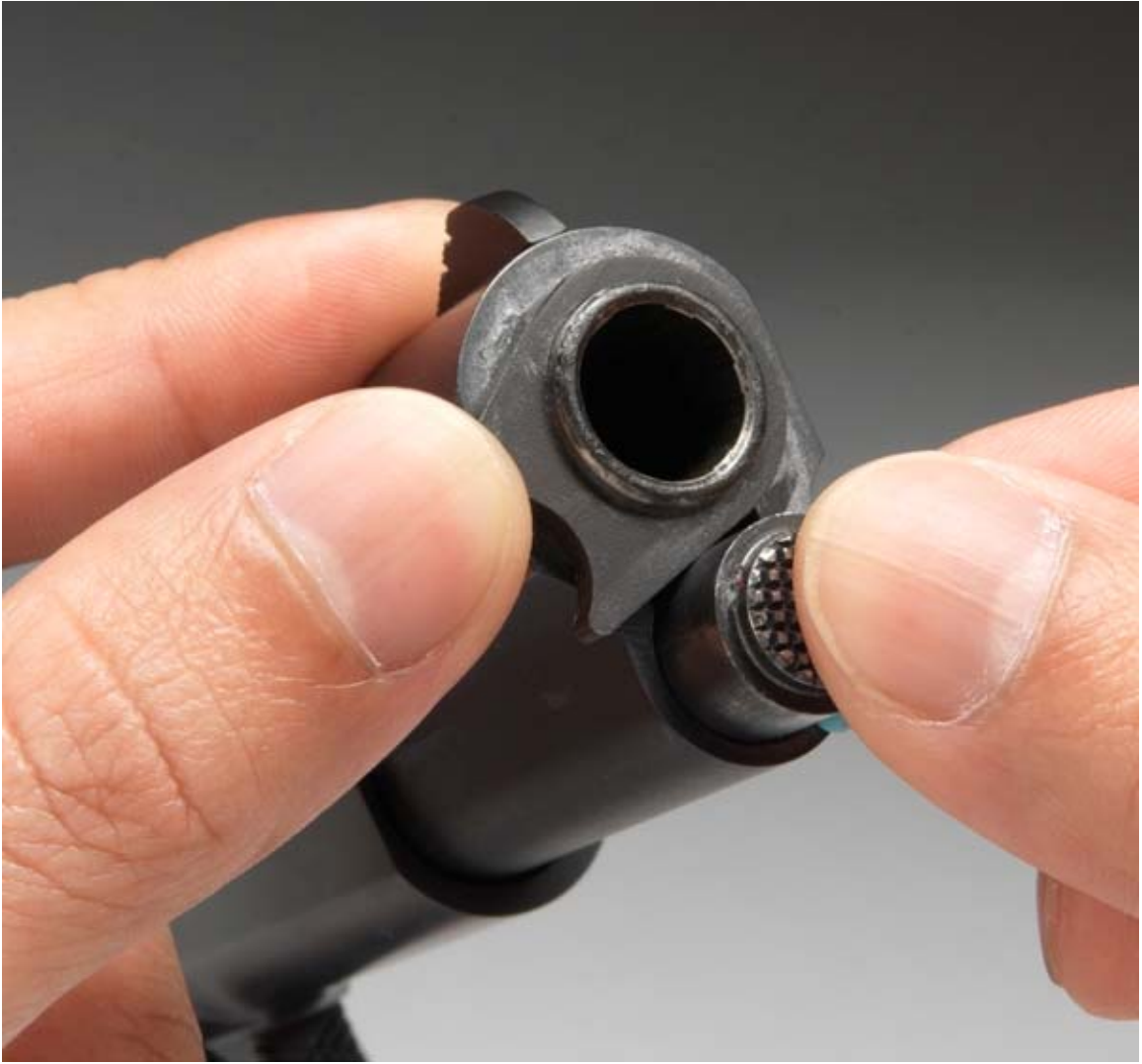
Figure 5. Remove the Recoil Spring Plug
