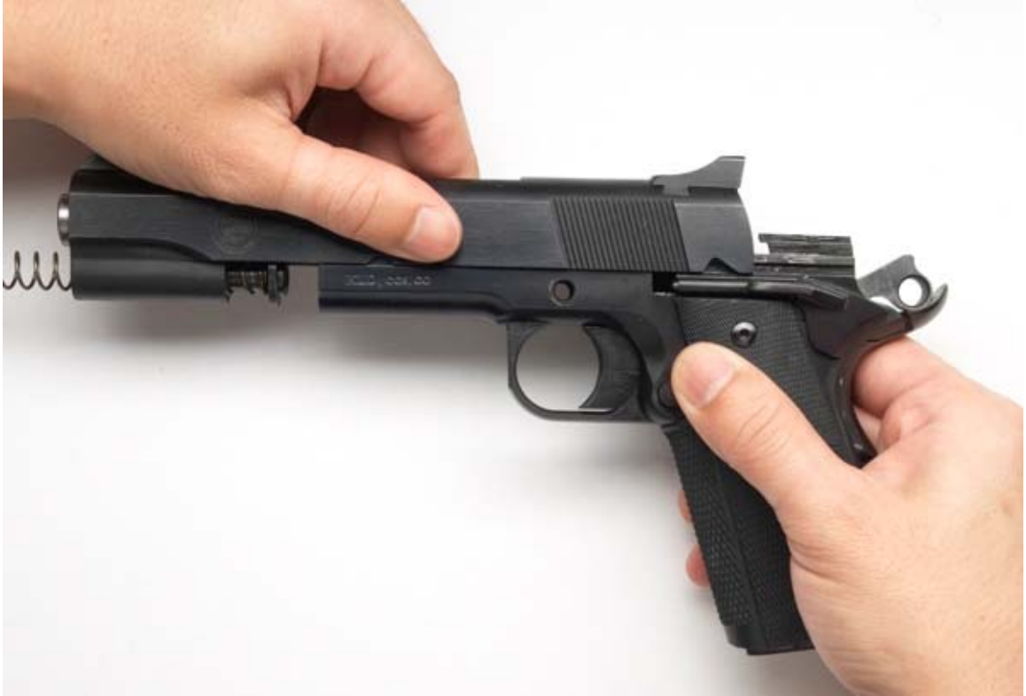
Fig. 7 Remove the Slide
